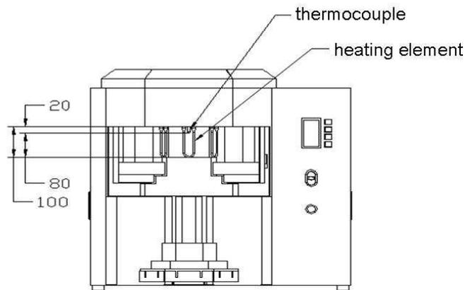
As already described in the section "**burn support**", the base area of the burn chamber is hexagonal and it has diagonals of 120 or 140 mm respectively and a square footage of 125 cm<sup>2</sup>.
