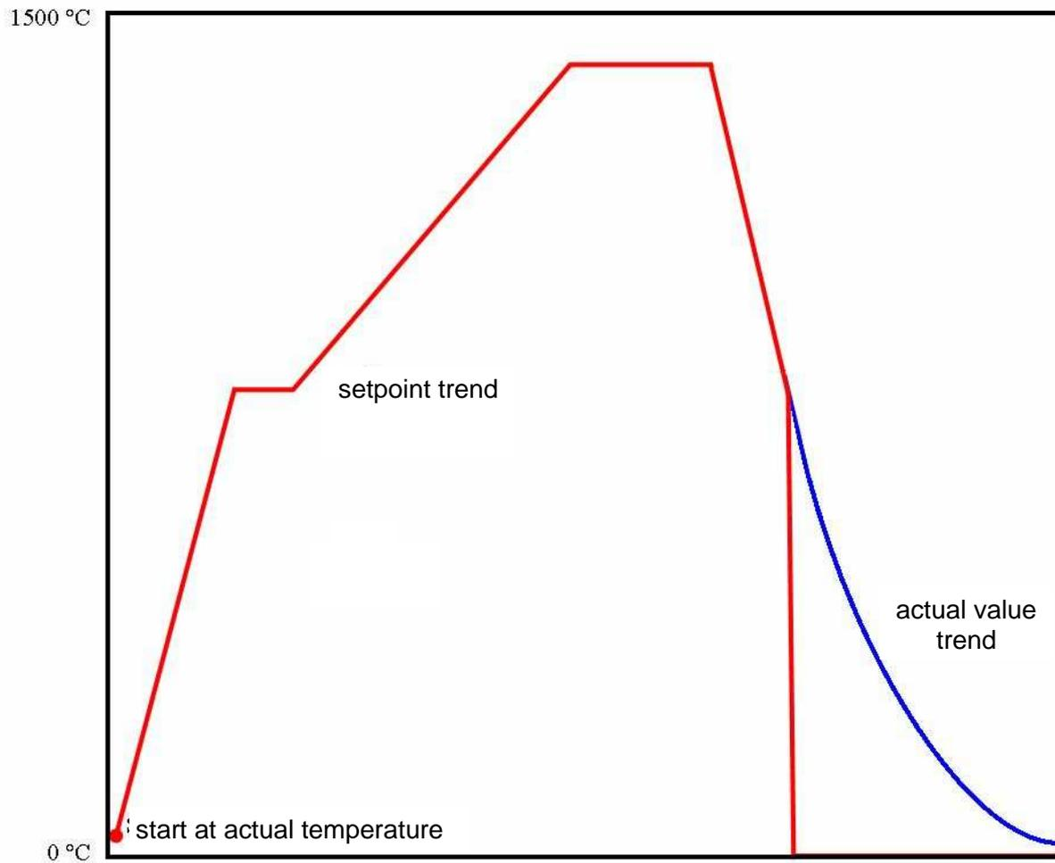
The factory-made sinter curve consists of an increasing ramp (heating up), a dwell time, another increasing ramp, another dwell time, a decreasing ramp (cooling down, controlled) and a skip (here cooling down, uncontrolled).
